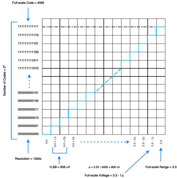
Figure 3 Quantization and Coding
