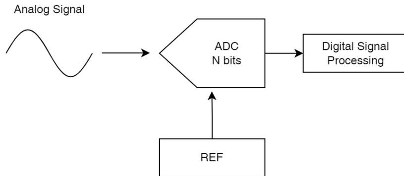
Figure 1 ADC Block Diagram
