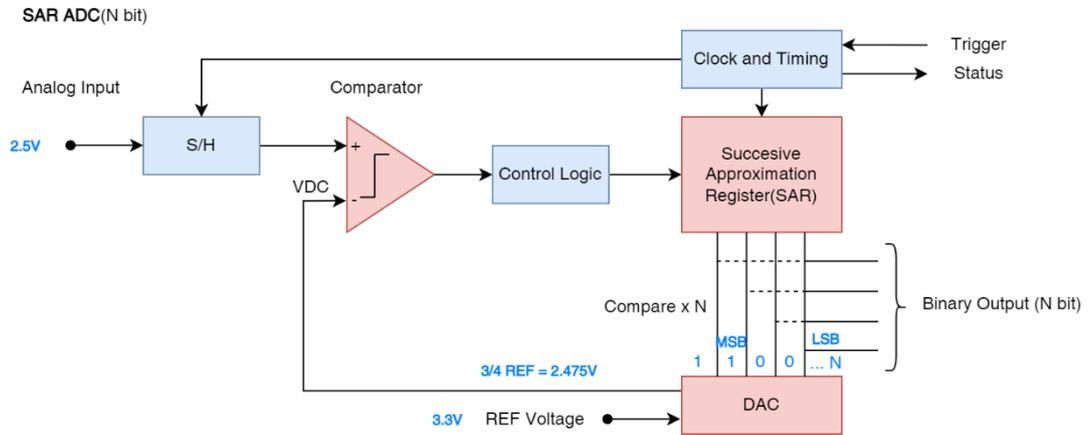
Figure 8 ADC Conversion Approximation Step 2
