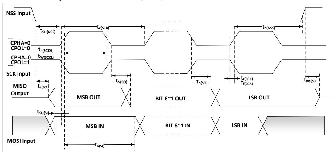
Figure 14 SPI timing diagram—slave mode and CPHA=1
