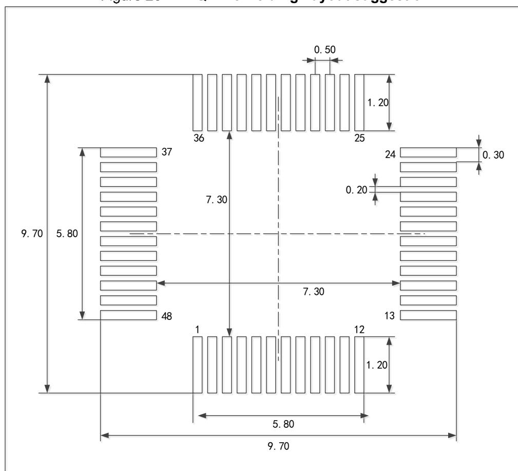
Note: Dimensions are in millimeters.
