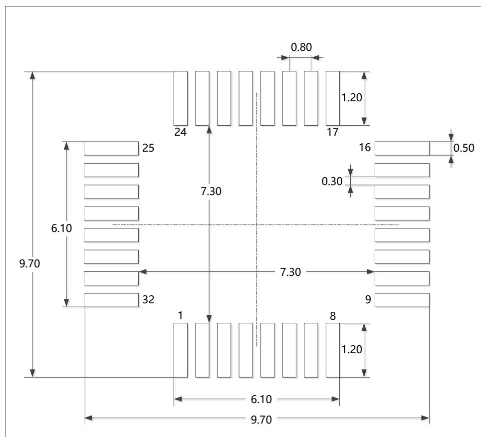
Note: Dimensions are in millimeters.
