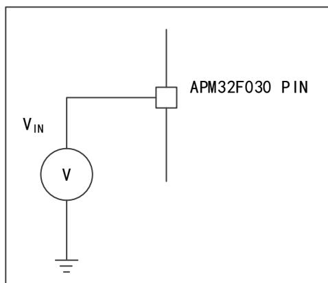
Figure 10 Current consumption measurement scheme
