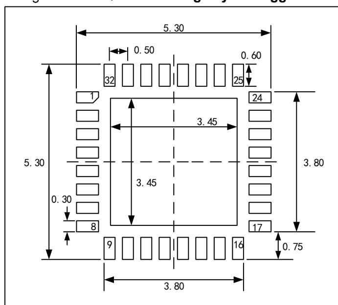
Figure 27 QFN32 Code specification
