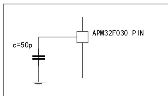
Figure 9 Pin input voltage measurement scheme
